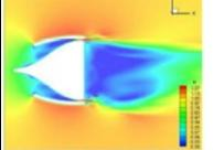
Figure 30. Instantaneous CFD Velocity contours for Jet2 bluff body model with high velocity passive jet pulsing, V<sub>Total</sub> = 30m/s Re=2.66×10<sup>5</sup>.
